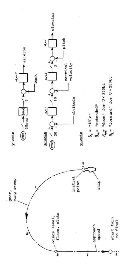
Figure 5. Features of the Break Maneuver Segment
