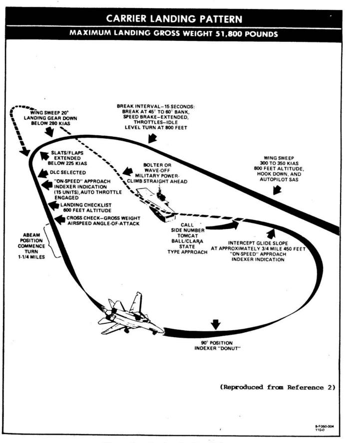
Figure 1. Carrier Landing Pattern
